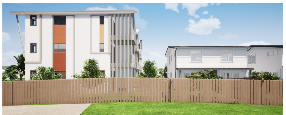
Artist's impression of the privacy screens on the three-storey building to reduce visibility from and to balconies
